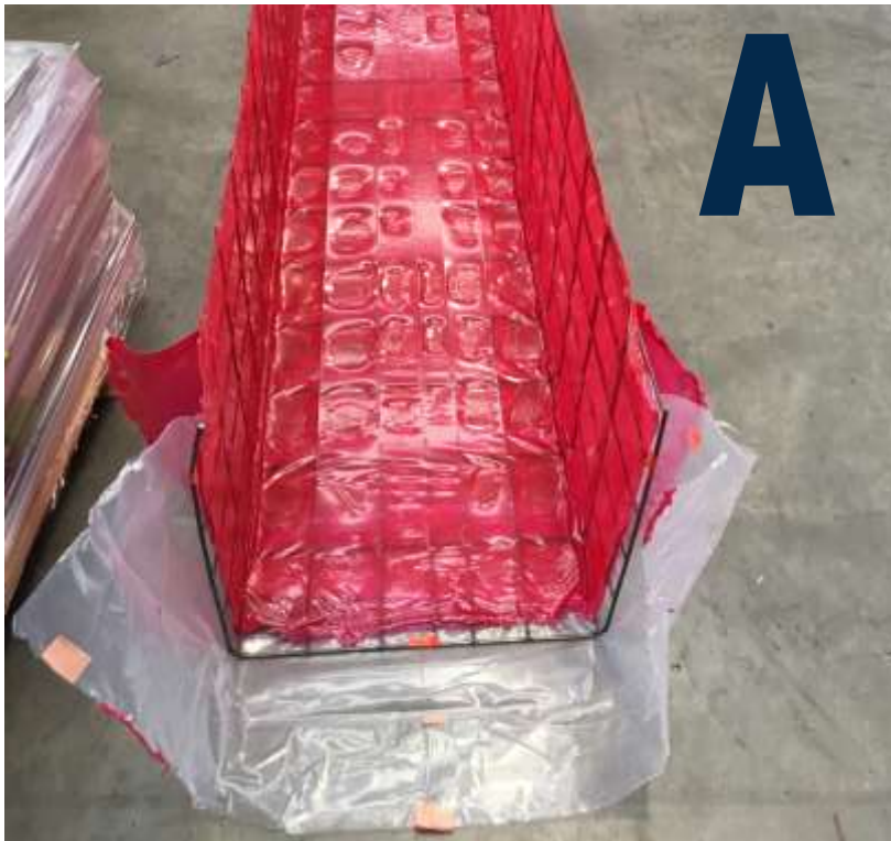
Type A: vapour membrane of .03mm virgin plastic and lapping all in one.
